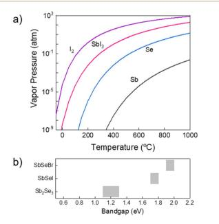
Fig. 1 (a) Vapor pressure of I<sub>2</sub>, Se and Sb as a function of temperature. (b) Bandgap range of Sb<sub>2</sub>Se<sub>3</sub>, SbSel and SbSeBr from literature.<sup>25–28</sup>
