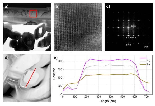
Fig. 5 TEM and EDX analysis of a Mo/SbSel sample prepared at 450 °C and 2 bar. (a) [001] HR-TEM cross-sectional image in the region marked with a red square. (b) HR-TEM image with high magnification. (c) FFT of image (b). (d) Cross-sectional image of an SbSel column severed transversally. (e) EDX profile mapping of the column in (d) along the red line.
