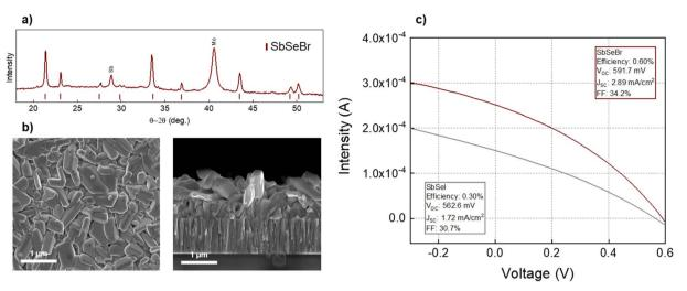
Fig. 8 (a) XRD pattern of the SLG/Mo/SbSeBr sample, (b) SEM top-view and cross-section micrographs of the SLG/Mo/SbSeBr sample, (c) intensity-voltage curves of SbSeBr and SbSeI prototype solar cells.
