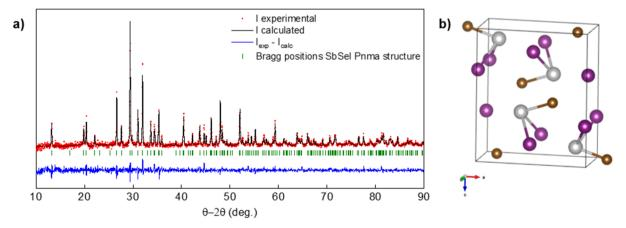
Fig. 4 (a) Experimental (red points) and Rietveld (black) refined patterns, along with the difference profile (blue curve) and Bragg reflections (green sticks) of SbSeI crystalline powder. (b) SbSeI unit cell structure obtained from XRD analysis, represented with the VESTA software: grey -Sb, brown - Se, purple - I.
