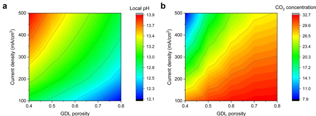
Fig. 1 Multiphysics simulation results of varying GDL porosity on the (a) local pH and (b)  $\text{CO}_2$  concentration at various cathodic current densities of 100, 200, 300, 400 and  $500 \text{ mA cm}^{-2}$ . A lower porosity is observed to result in a higher local pH and lower  $\text{CO}_2$  concentration. Detailed results can be found in the ESI (Fig. S1–S6†).
