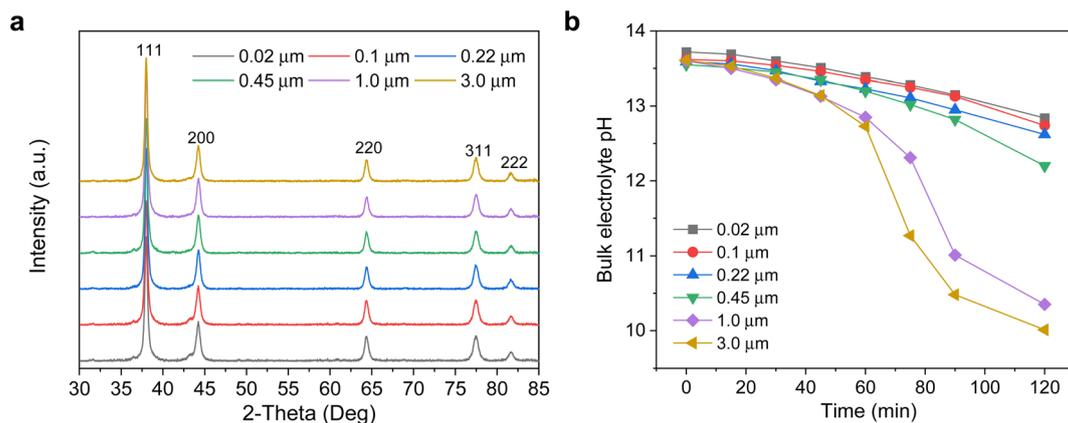
Fig. 3 (a) XRD spectra of Ag sputtered onto PTFE substrates with various pore sizes. (b) Evolution of the bulk electrolyte pH over a 120 min period, with no current applied to the system. 15 ml of 1 M KOH was used as the electrolyte and was continuously recirculated through the electrochemical cell using a peristaltic pump.
