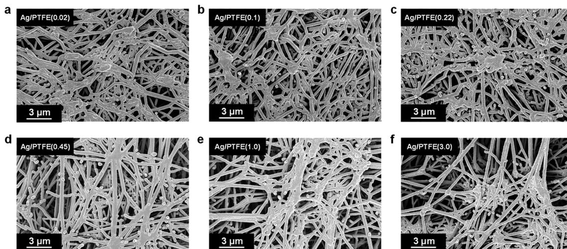
Fig. 2 SEM images of hydrophobic PTFE substrates of various pore sizes coated with 325 nm of Ag using sputter deposition. The pore sizes are: (a)  $0.02 \mu\text{m}$ , (b)  $0.1 \mu\text{m}$ , (c)  $0.22 \mu\text{m}$ , (d)  $0.45 \mu\text{m}$ , (e)  $1.0 \mu\text{m}$  and (f)  $3.0 \mu\text{m}$ . Digital photographs (Fig. S7†) and more SEM images (Fig. S8–S10†) of the samples can be found in the ESI.†
