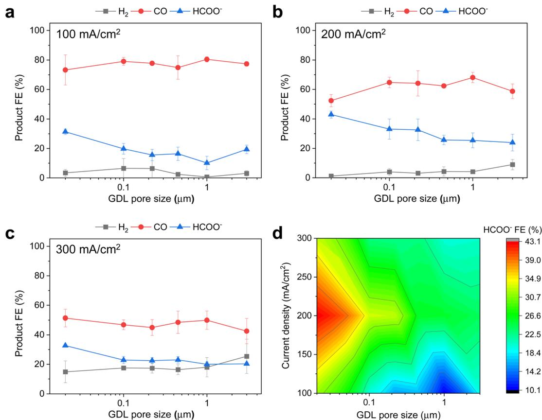
Fig. 4 Electrochemical  $\text{CO}_2$  reduction FE results with 1 M  $\text{KHCO}_3$  as the electrolyte. (a), (b) and (c) show the product FE data for Ag/PTFE as a function of GDL pore size under cathodic current densities of 100, 200 and 300 mA  $\text{cm}^{-2}$  respectively. (d) Is the corresponding color contour map of the  $\text{HCOO}^-$  FE data for Ag/PTFE as a function of current density and GDL pore size. More data available in the ESI (Fig. S16†).
