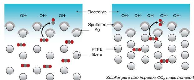
Scheme 1 CO<sub>2</sub> mass transport through the gas diffusion layer is slower with a smaller GDL pore size. This results in a higher local pH, which then induces a higher selectivity towards formate. Note: items in the schematic are not drawn to scale.
