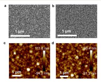
Fig. 1 Top-view SEM and AFM images of  $In_2S_3$  buffer layers (a and c) without  $InCl_3$  post-treatment and (b and d) with post-treatment by using 0.02 g mL<sup>-1</sup>  $InCl_3$ .
