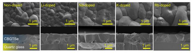
Fig. 1 Surface/cross-section SEM images of non-doped and alkali-(i.e., Li, Na, K, and Rb) doped CBGTSe films deposited on quartz glass substrates. All scale bars represent 1 µm. Note that the alkali-doping was achieved by pre-depositing approximately 4-nm-thick layers of alkali fluoride (e.g., KF). Cross-section images were acquired after depositing  $\sim$ 5 nm of Au to avoid surface charging.
