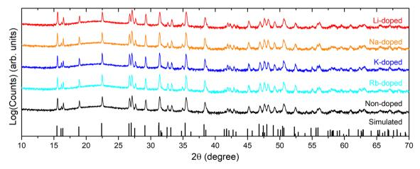
Fig. 2 XRD patterns for CBGTSe films with different dopants, plotted on a log scale to accentuate any possible impurities. The simulated XRD stick pattern for CBGTSe (x = 0.7) was simulated using CrystalDiffract software with lattice parameters adapted from Wessler et al. 48 XRD patterns of the doped CBGTSe films exhibit only the simulated peaks of the main phase, which excludes significant formation of secondary phases.
