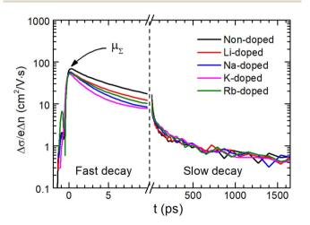
Fig. 6 THz photoconductivity transient curves obtained from nondoped and alkali-doped (pre-deposited with 4 nm of alkali fluoride layers) CBGTSe films, showing fast-/slow-decaying components, and terahertz sum mobilities ( $\mu_{\Sigma}$ ).
