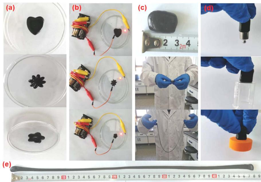
Fig. 6 (a) Digital photograph of the plasticity of APC-PVA@ZnCl<sub>2</sub> materials; (b) electrical conductivity; (c) stretchability; (d) adhesion; (e) tensile length.
