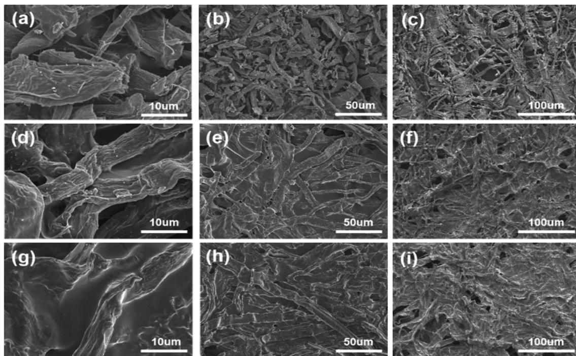
Fig. 2 The SEM images of (a–c) APC, (d–f) APC@PVA, (g–i) APC-PVA@ZnCl<sub>2</sub> under different magnifications.
