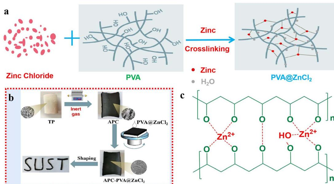
Fig. 1 (a) Configuration mechanism of  $\text{PVA@ZnCl}_2$  solution. (b) The preparation process of  $\text{APC-PVA@ZnCl}_2$  with good plasticity. (c) The cross-linking mechanism between PVA and  $\text{Zn}^{2+}$ .
