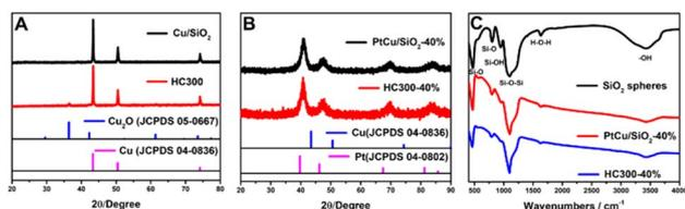
Fig. 1 (A) XRD patterns of Cu/SiO<sub>2</sub> and HC300; (B) XRD patterns of PtCu/SiO<sub>2</sub>-40% and HC300-40%; (C) FTIR spectra of SiO<sub>2</sub> spheres, PtCu/SiO<sub>2</sub>-40% and HC300-40%.
