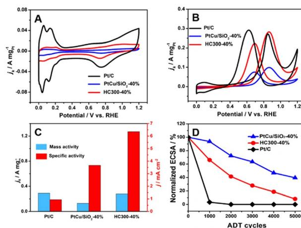
Fig. 4 (A) CVs of commercial Pt/C (20 wt% Pt), PtCu/SiO<sub>2</sub>-40%, and HC300-40%; (B) MOR activity; (C) mass and specific activities obtained from MOR results; (D) accelerating durability tests (ADT) of commercial Pt/C (20 wt% Pt), PtCu/SiO<sub>2</sub>-40%, and HC300-40%.
