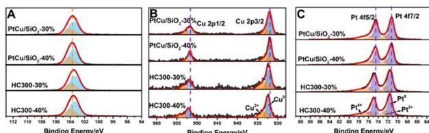
Fig. 3 XPS spectra of the Si 2p (A), Cu 2p (B), and Pt 4f (C) orbitals of PtCu/SiO<sub>2</sub>-30%, HC300-30%, PtCu/SiO<sub>2</sub>-40% and HC300-40%.
