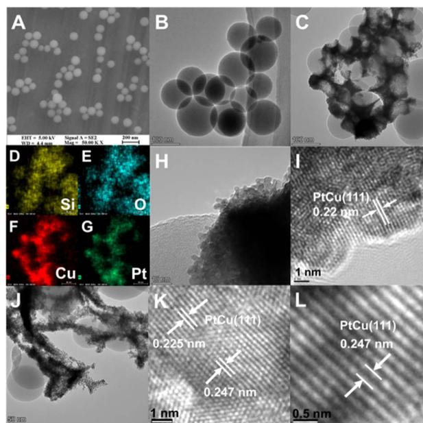
Fig. 2 (A) SEM image of SiO<sub>2</sub> nanospheres; (B) TEM image of SiO<sub>2</sub> nanospheres; (C–G) TEM and EDS images of PtCu/SiO<sub>2</sub>-40%; (H) magnification of a specific region of (C); (I) High resolution image of PtCu/SiO<sub>2</sub>-40%, showing the magnification of a specific region of (H); (J) TEM image of HC300-40%; (K and L) high resolution images of HC300-40%.
