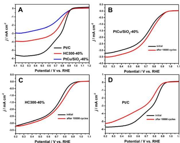
Fig. 5 (A) The ORR curves of Pt/C, HC300-40%, and PtCu/SiO<sub>2</sub>-40%; the changes in ORR polarization curves under potential cycling (scan rate 10 mV s<sup>-1</sup>, O<sub>2</sub> saturated) of PtCu/SiO<sub>2</sub>-40% (B), HC300-40% (C) and Pt/C (D).
