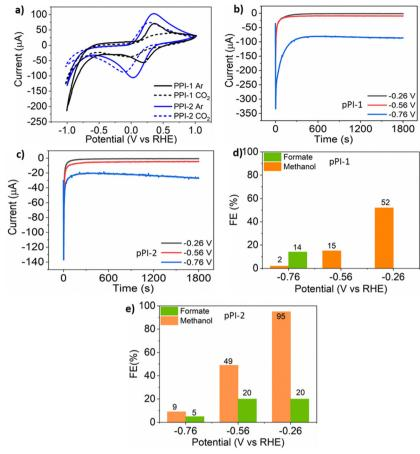
Fig. 3 (a) Cyclic voltammogram of pPI-1 and pPI-2 in the applied potential range from -1-1 V vs. RHE, scan rate 20 mV s<sup>-1</sup>, 20 cycles, (b) and (c) chronoamperometry studies (vs. RHE) of pPI-1 and pPI-2, respectively in CO2-saturated electrolytes, and (d) and (e) highest obtained faradaic efficiency of pPI-1 and pPI-2, respectively in CO<sub>2</sub> saturated electrolytes for 30 min.
