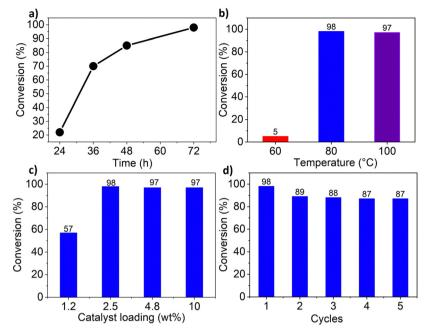
Fig. 2 (a) Time-dependent percentage conversion of ECH at 80 °C for pPI-1. (b) Temperature-dependent conversion for cycloaddition of CO<sub>2</sub> to ECH for pPI-1. (c) pPI-1 catalyst loading for cycloaddition of CO<sub>2</sub> to ECH at 80 °C. (d) Recycling test of pPI-1 for the cycloaddition of CO<sub>2</sub> to ECH at 80 °C
