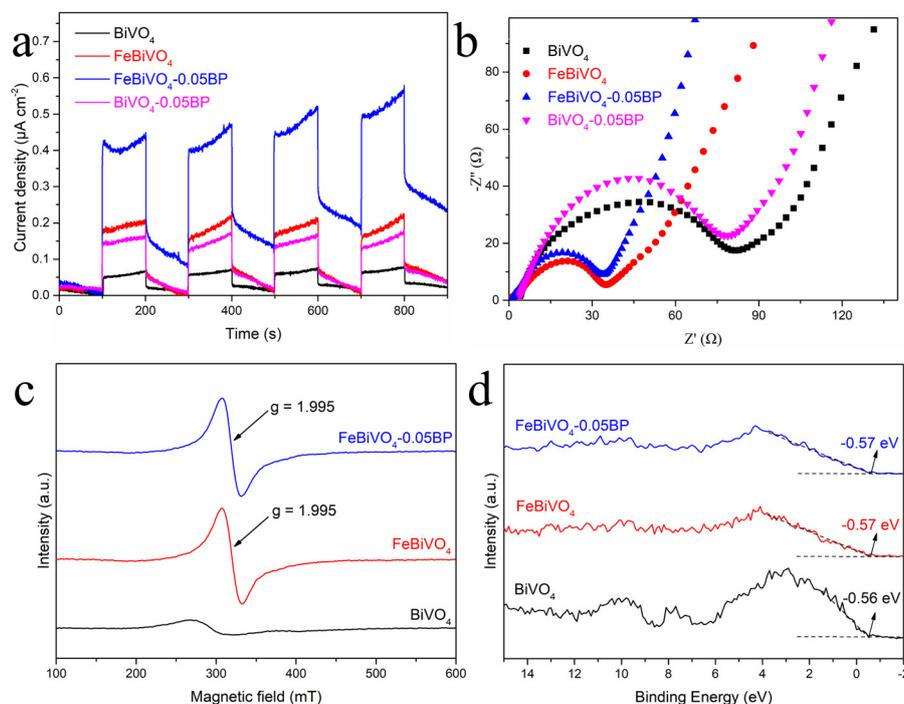
**Fig. 7** (a) Photocurrent response and (b) electrochemical impedance spectroscopy (EIS) tests of  $\text{BiVO}_4$ ,  $\text{FeBiVO}_4$ ,  $\text{BiVO}_4\text{-0.05BP}$  and  $\text{FeBiVO}_4\text{-0.05BP}$ ; (c) EPR spectra and (d) XPS valence state spectra of  $\text{BiVO}_4$ ,  $\text{FeBiVO}_4$  and  $\text{FeBiVO}_4\text{-0.05BP}$ .
