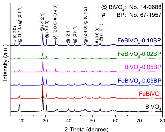
Fig. 1 XRD patterns of different samples: BiVO<sub>4</sub>, FeBiVO<sub>4</sub>, BiVO<sub>4</sub>-0.05BP, FeBiVO<sub>4</sub>-0.05BP, FeBiVO<sub>4</sub>-0.02BP and FeBiVO<sub>4</sub>-0.10BP.
