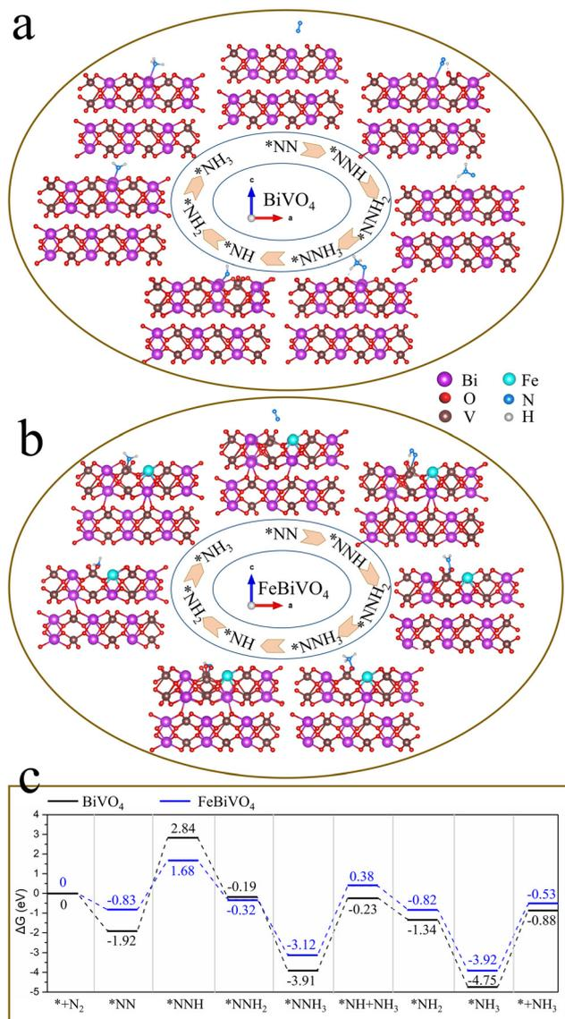
**Fig. 6** Optimized structures of reaction intermediates in a distal mechanism: (a) BiVO<sub>4</sub> and (b) FeBiVO<sub>4</sub>; (c) Gibbs free energy profiles of nitrogen reduction over BiVO<sub>4</sub> and FeBiVO<sub>4</sub> catalysts by a distal mechanism.
