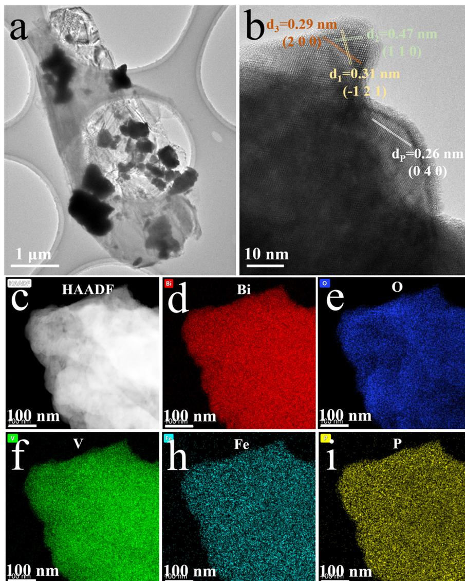
Fig. 3 (a) TEM and (b) High-resolution TEM images of  $\text{FeBiVO}_4\text{-0.05BP}$ ; (c) HAADF-STEM image and corresponding EDS mapping: (d) Bi, (e) O, (f) V, (h) Fe, (i) P.
