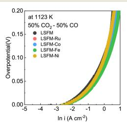
Fig. 5 (a and b) The Tafel plot (fitted with an overpotential of 0.1-0.2 V) of the LSFM and metal-infiltrated LSFM electrodes (Co, Fe, Ni, and Ru) in the CO<sub>2</sub> electrolysis at 1123 K.
