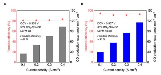
Fig. 7 Faradaic efficiency of the cell with (a) bare LSFM, and (b) LSFM-Fe electrode with a CO<sub>2</sub>: CO gas (50:50) mixture at 1123 K.
