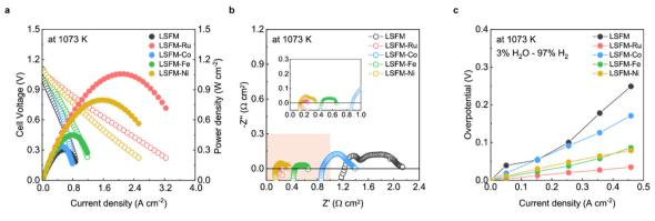
Fig. 3 (a) The I-V curves and (b) the impedance data of single cells of LSFM and infiltrated LSFM electrodes (Co, Fe, Ni, and Ru) at 1073 K under  $H_2O: H_2$  (3%:97%. (c) The polarization overpotential is calculated from the impedance data.
