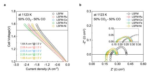
Fig. 4 (a) The  $CO_2$  electrolysis performance with the infiltrated LSFM electrode feeding  $CO_2$ : CO (50:50) at 1123 K. (b) Total impedance spectra of the cell with the infiltrated LSFM electrode at 1123 K.
