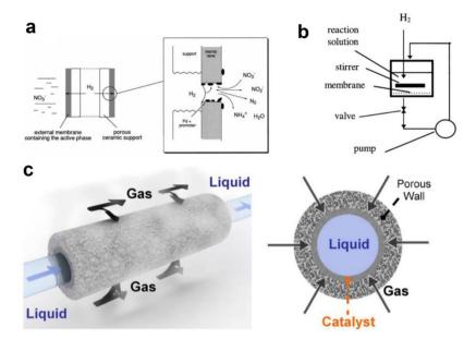
Fig. 2 (a) Schematic illustration of a catalytic membrane reactor for nitrate and nitrite reduction. (b) The flow-through configuration of a catalytic membrane reactor.<sup>49</sup> Copyright 2013, American Chemical Society. (c) The gas-liquid-solid contact in a porous ceramic reactor.<sup>50</sup> Copyright 2011, Elsevier.
