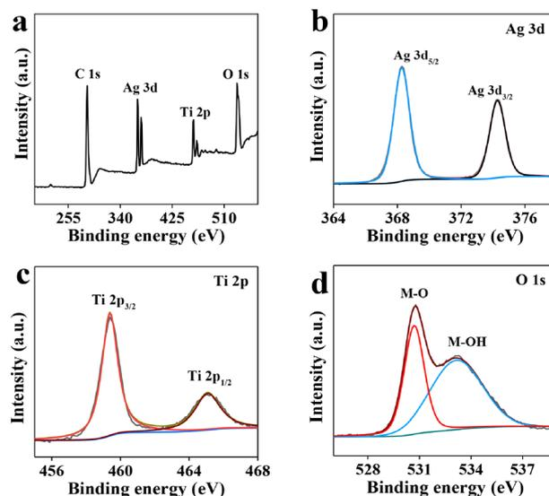
**Fig. 2** (a) XPS survey spectrum, and high resolution XPS spectra in the (b) Ag 3d, (c) Ti 2p, and (d) O 1s regions of Ag@TiO<sub>2</sub>.
