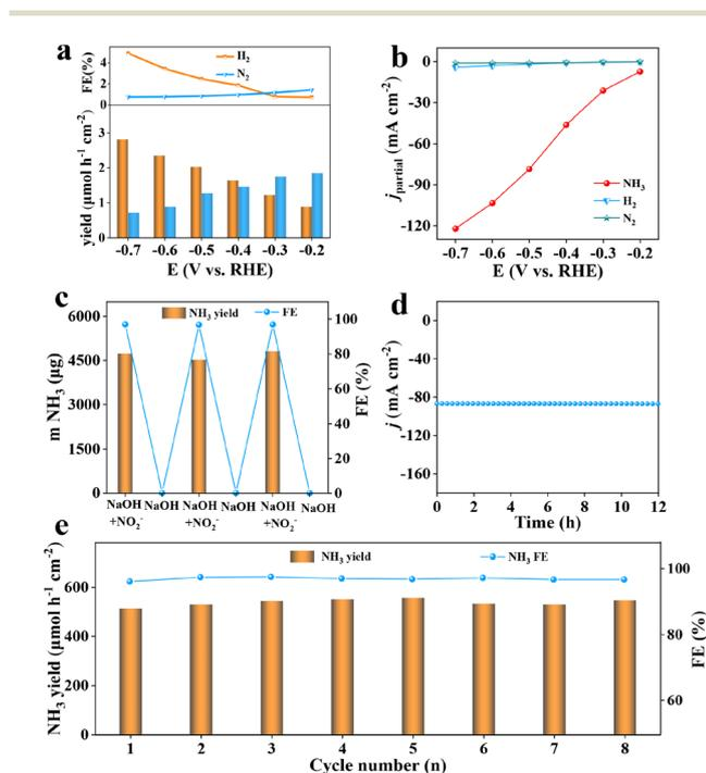
**Fig. 4** (a) Yields and FEs of N<sub>2</sub> and H<sub>2</sub> of Ag@TiO<sub>2</sub>/TP at different potentials. (b) *j*<sub>partial</sub> of NH<sub>3</sub>, N<sub>2</sub>, and H<sub>2</sub> of Ag@TiO<sub>2</sub>/TP at different potentials. (c) NH<sub>3</sub> yields and FEs of Ag@TiO<sub>2</sub>/TP during the alternating cycling tests. (d) Time-dependent current density curve during 12 h electrolysis of Ag@TiO<sub>2</sub>/TP at -0.5 V. (e) Recycling tests of Ag@TiO<sub>2</sub>/TP at -0.5 V.
