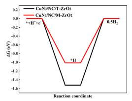
Fig. 5 DFT-calculated free energy diagrams of the HER on CuN<sub>3</sub>/NC/  $T-ZrO_2(101)$  and  $CuN_3/NC/M-ZrO_2(-111)$  at a potential (U) = 0 V.
