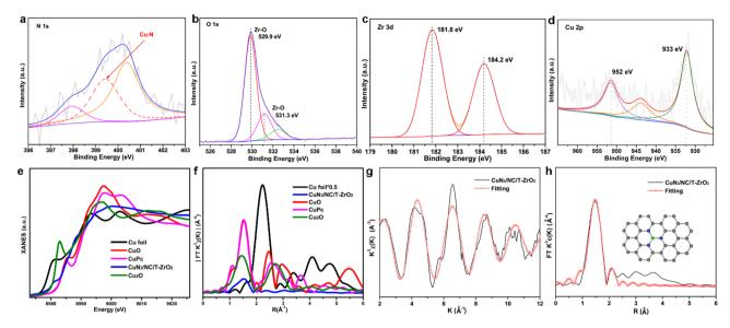
Fig. 2 (a-d) XPS spectra of CuN<sub>3</sub>/NC/T-ZrO<sub>2</sub>: N 2p, O 1s, Zr 3d, and Cu 2p, respectively. (e) Cu K-edge data of Cu foil, CuO, CuPc, Cu<sub>2</sub>O, and  $\text{CuN}_3/\text{NC/T-ZrO}_2$ . (f) Fourier transform (FT)  $k^3$ -weighted EXAFS profiles at the Cu k-edge. (g) Fitting curves. (h) EXAFS R space fitting curves of CuN<sub>3</sub>/NC/T-ZrO<sub>2</sub>.
