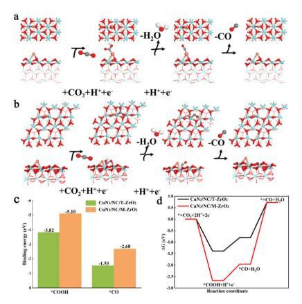
Fig. 4 (a) CO<sub>2</sub>RR processes on CuN<sub>3</sub>/NC/T-ZrO<sub>2</sub>(101) and (b) CuN<sub>3</sub>/NC/M-ZrO<sub>2</sub>(-111). (c) Calculated binding energies (in eV) on CuN<sub>3</sub>/NC/ T-ZrO<sub>2</sub>(101) and CuN<sub>3</sub>/NC/M-ZrO<sub>2</sub>(-111). (d) Calculated free energy diagrams of the CO<sub>2</sub>RR on CuN<sub>3</sub>/NC/T-ZrO<sub>2</sub>(101) and CuN<sub>3</sub>/NC/M-ZrO<sub>2</sub>(-111).
