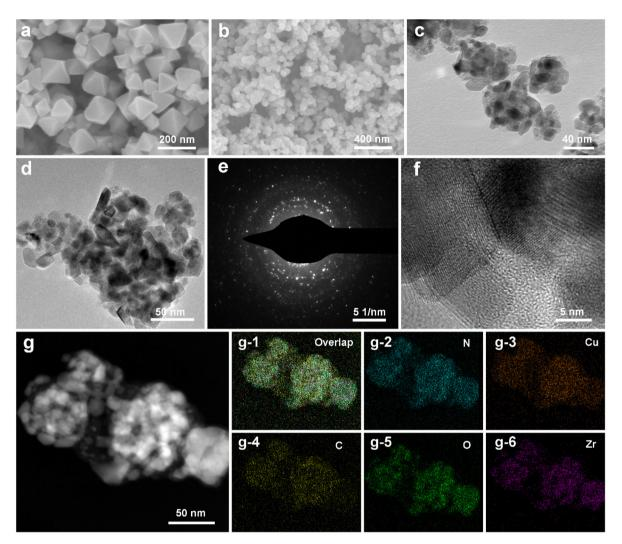
Fig. 1 (a) SEM image of Cu-UIO-66-NH<sub>2</sub>. (b and c) SEM and TEM images of CuN<sub>3</sub>/NC/T-ZrO<sub>2</sub>. (d-f) TEM, selected area electron diffraction (SAED), and STEM images of CuN<sub>3</sub>/NC/T-ZrO<sub>2</sub>. (g) EDS elemental mapping of CuN<sub>3</sub>/NC/T-ZrO<sub>2</sub>.
