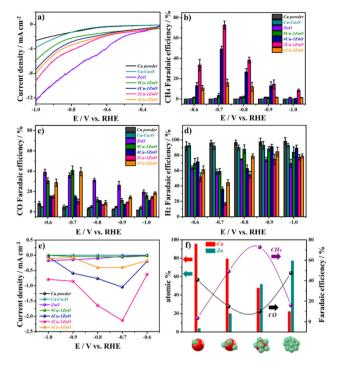
Fig. 3 (a) Linear sweep voltammetry curves, (b) CH<sub>4</sub> faradaic efficiency, (c) CO faradaic efficiency, and (d) H2 faradaic efficiency of Cu powder, Cu-Cu<sub>2</sub>O, ZnO, and Cu-ZnO with different Cu: Zn ratios. (e) CH<sub>4</sub> partial current density of different catalysts. (f) Relationship between the performance, components, and morphology of Cu-ZnO catalysts.
