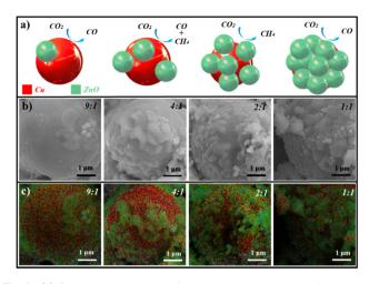
Fig. 1 (a) Schematic diagrams of the designed heterointerface structures. Red and green balls represent metal Cu and ZnO, respectively. (b) SEM images and (c) overlap mapping pictures of the Cu-ZnO catalysts with different heterointerfaces. The Cu:Zn ratios were 9:1, 4:1, 2:1, and 1:1, respectively. Red and green areas represent the element distribution of Cu and Zn, respectively. The ratios were acquired from ICP tests.
