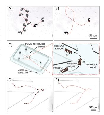
Fig. 3 (A and B) Time-lapse images showing the trajectory of a PiezoBOT under magnetic manipulation in DI water. (C) Scheme of the PDMS microfluidic device. (D and E) Trajectory of a PiezoBOT under magnetic manipulation in PBS solution in a microfluidic vasculature model.
