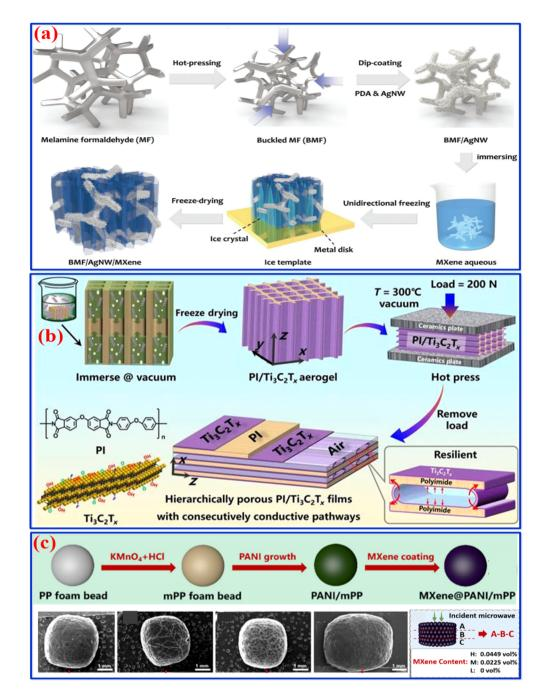
Fig. 8 (a) Buckled melamine formaldehyde sponges coated with AgNW/MXene hybrid hierarchical composite. Reproduced from ref. 148 with permission from the Royal Society of Chemistry, © 2019. (b) Hierarchically porous  $PI/Ti_3C_2T_x$  composite. Reproduced from ref. 108 with permission from the Authors, © 2021. (c) MXene network decorated with polypropylene foam beads. Reproduced from ref. 149 with permission from Elsevier Ltd., © 2020.
