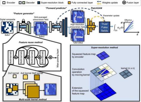
Fig. 11 The architecture of DGNet. The DGNet is composed of two generators the G-1 and the G-2. The G-1 generates a grid-averaged image from the shape of the digital composite, and the G-2 generates a high-resolution stress/strain field image. The DGNet is trained adversarially, and effective stiffness is estimated from the generated high-resolution image. Reproduction with permission from ref. 105. Copyright (2023) Elsevier.
