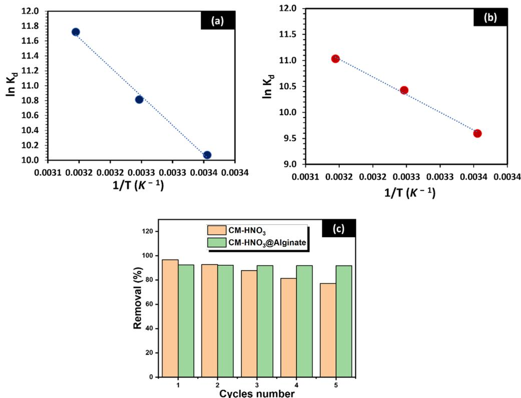
Fig. 6 The van't Hoff plot for MB adsorption onto (a) CM-HNO<sub>3</sub> and (b) CM-HNO<sub>3</sub>@Alginate; (c) the reusability study of CM-HNO<sub>3</sub> and CM-HNO<sub>3</sub>@Alginate.
