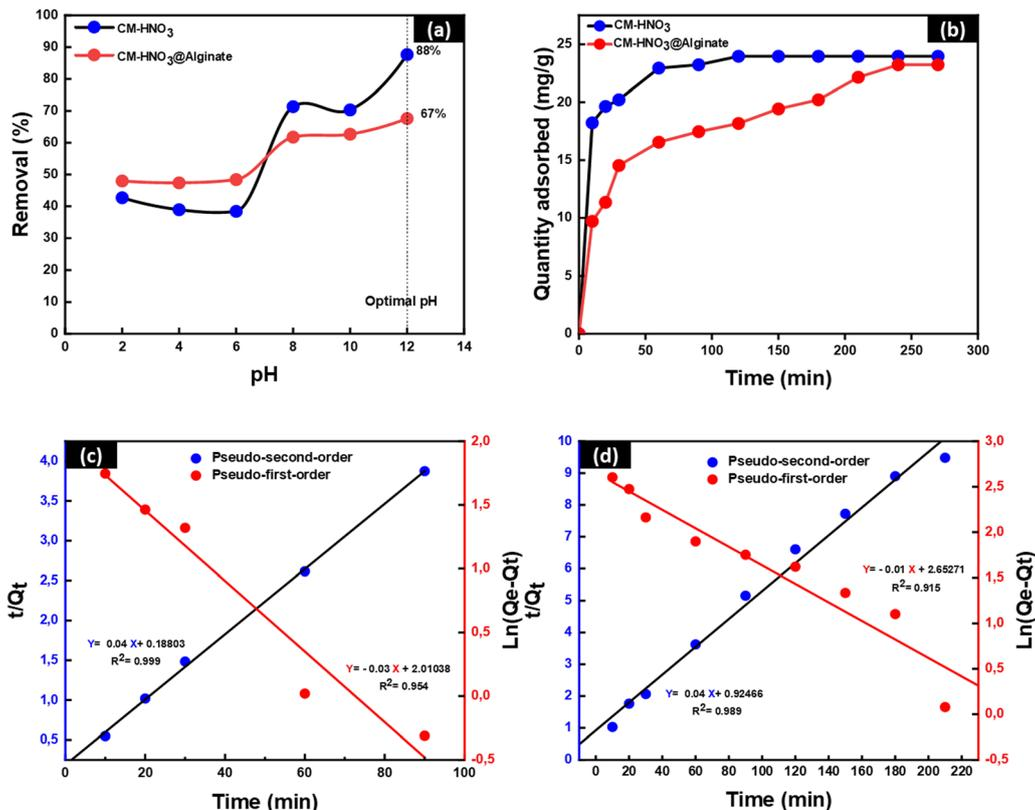
Fig. 4 The effect of (a) pH and (b) contact time on the adsorption of MB. Adsorption kinetics of MB on (c) CM-HNO<sub>3</sub> and (d) CM-HNO<sub>3</sub>@Alginate.
