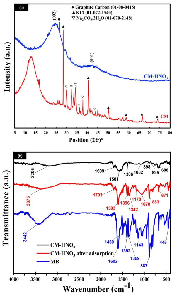
Fig. 1 (a) The XRD patterns of CM and CM-HNO<sub>3</sub>; (b) the FTIR spectra of CM-HNO<sub>3</sub>, CM-HNO<sub>3</sub> after adsorption, and MB.
