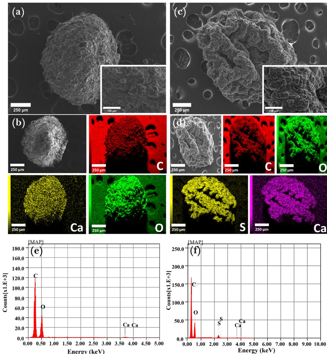
Fig. 3 The SEM and mapping analyses of CM-HNO<sub>3</sub>@Alginate beads (a), (b), (e) before and (c), (d), (f) after MB adsorption.
