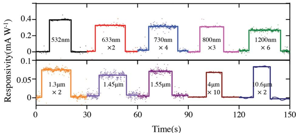
Fig. 8 Photocurrent response of the MoTe<sub>2</sub> device at different excitation wavelengths. Reprinted with permission from ref. 110. Copyright 2018, Wiley.
