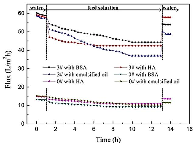
Fig. 21 The time-dependent flux of the PIP-TMC NF membrane (#0) and the GQD/PIP-TMC TFN membrane (#3) during the filtration of HA, BSA, and emulsified oil solutions.<sup>161</sup> Reprinted with permission from ref. 161. Copyright (2018) Elsevier.
