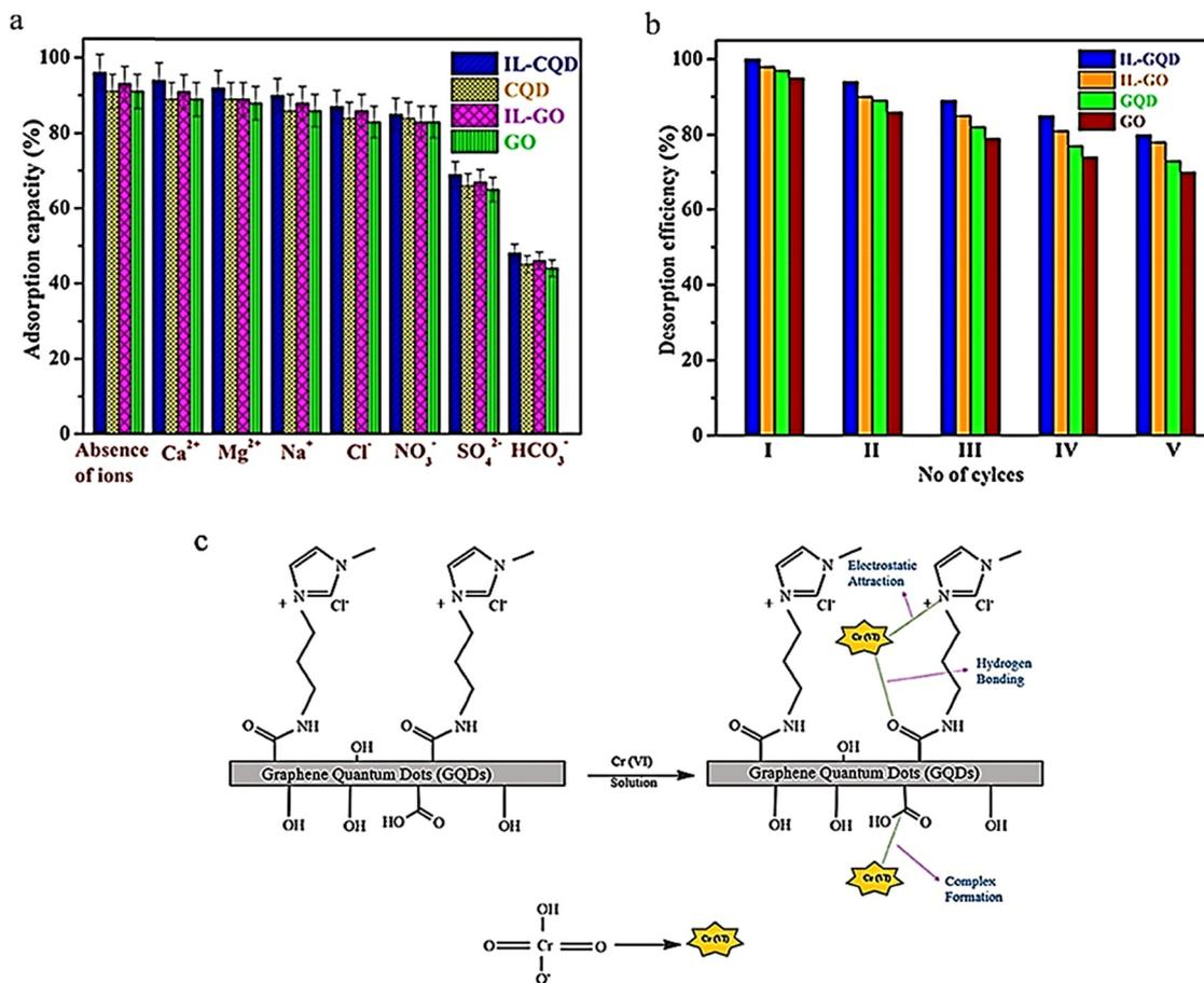
Fig. 14 Effect of competing Cr<sup>6+</sup> ion adsorption with adsorbents GQD and IL-GQD (a), desorption of the adsorbents IL-GO, IL-GQD, GO, and GQD (b), and acceptable Cr<sup>6+</sup> adsorption mechanism of the IL-GQD adsorbent (c). (a) and (c) Reprinted with permission from ref. 127 Copyright (2019) American Chemical Society. (b) Reprinted with permission from ref. 11. Copyright (2021) Elsevier.
