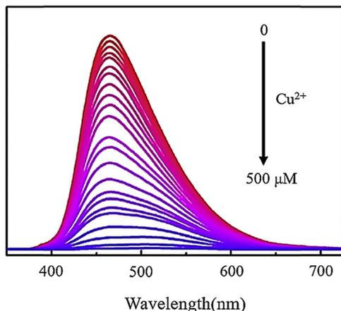
Fig. 16 Fluorescence spectra of N-GQDs, including Cu<sup>2+</sup> with different concentrations from 0 to 500 μM. Reprinted with permission from ref. 145. Copyright (2020) Elsevier.
