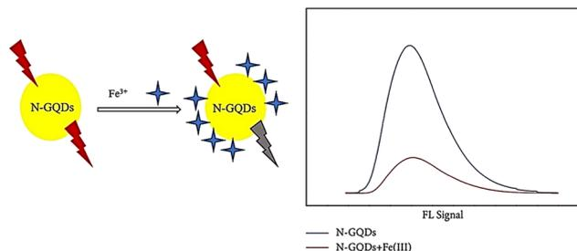
Fig. 17 Quenching N-GQD fluorescence with iron ions. Reproduced with permission from ref. 147. Copyright (2019) Hindawi.
