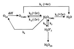
Fig. 1 Schematic diagram of the ORR process under acid conditions. 16
