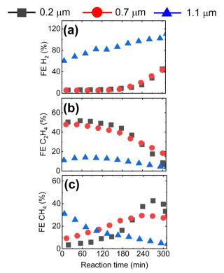
Fig. 4 Faradaic efficiency for (a)  $H_2$ , (b)  $C_2H_4$ , and (c)  $CH_4$  at 200 mA cm $^{-2}$  as a function of time for GDEs with mean pore size 0.2  $\mu$ m, 0.7  $\mu$ m, and 1.1  $\mu$ m.
