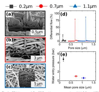
Fig. 1 SEM images of Cu-GDEs with mean pore size of (a) 0.2  $\mu m$  (15% PDVF-HFP), (b) 0.7  $\mu m$  (30% PDVF-HFP), and (c) 1.1  $\mu m$  (32% PDVF-HFP), and (d) corresponding pore size distribution, and (e) water entry pressure vs. mean pore size. Note the different scale bars in the SEM images. The obtained fibers (darker contrast) are coated with Cu (lighter contrast) close to the top surface of the GDE.
