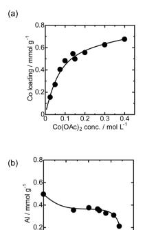
Fig. 2 (a) Relationship between the Co loading of Co/MFI(52N) and concentration of Co(OAc)2. (b) Relationship between Co loading and the Al concentration of Co/MFI(52N).
