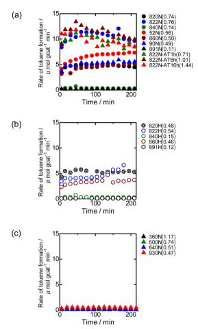
Fig. 9 Time course change of the toluene formation rate over Co loaded on different kinds of zeolite supports: (a) NH<sub>4</sub>-form MFI, (b) H-form MFI, and (c) zeolites other than MFI. The Co/MFI catalysts were prepared using a 200 mmol L<sup>-1</sup> Co(OAc)<sub>2</sub> solution at 343 K for 4 h. The numbers in the parentheses indicate the loading of Co (mmol  $g^{-1}$ ).
