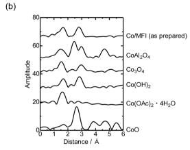
Fig. 1 Co K-edge (a) XANES and (b) EXAFS-FT of Co/MFI(52N) (Co: 0.5 mmol g<sup>-1</sup>) and reference compounds measured at 298 K. Fourier transform range: 3-13 Å<sup>-1</sup>.
