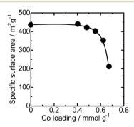
Fig. 7 Specific surface area plotted as a function of Co loadings of Co/MFI(52N).
