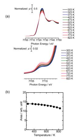
Fig. 3 (a) Co K-edge XANES of Co/MFI(52N) (Co: 0.5 mmol g<sup>-1</sup>) measured under a N2 flow from 303 to 823 K measured under in situ conditions. (b) White line area in Co K-edge XANES of Co/MFI(52N) plotted as a function of the treatment temperature.
