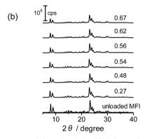
Fig. 6 XRD patterns of Co-unloaded MFI(52N) and Co/MFI(52N). (a) The as-prepared and (b) 773 K-treated samples. The numbers indicate the Co loading (mmol  $\rm g^{-1}$ ).
