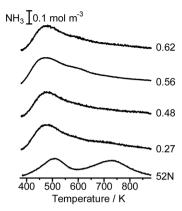
Fig. 5  $NH_3$  TPD profile of unloaded MFI(52N) and Co/MFI(52N). The samples were treated in an  $N_2$  flow at 773 K prior to the TPD measurement. The numbers indicate the loading of Co (mmol  $g^{-1}$ ).
