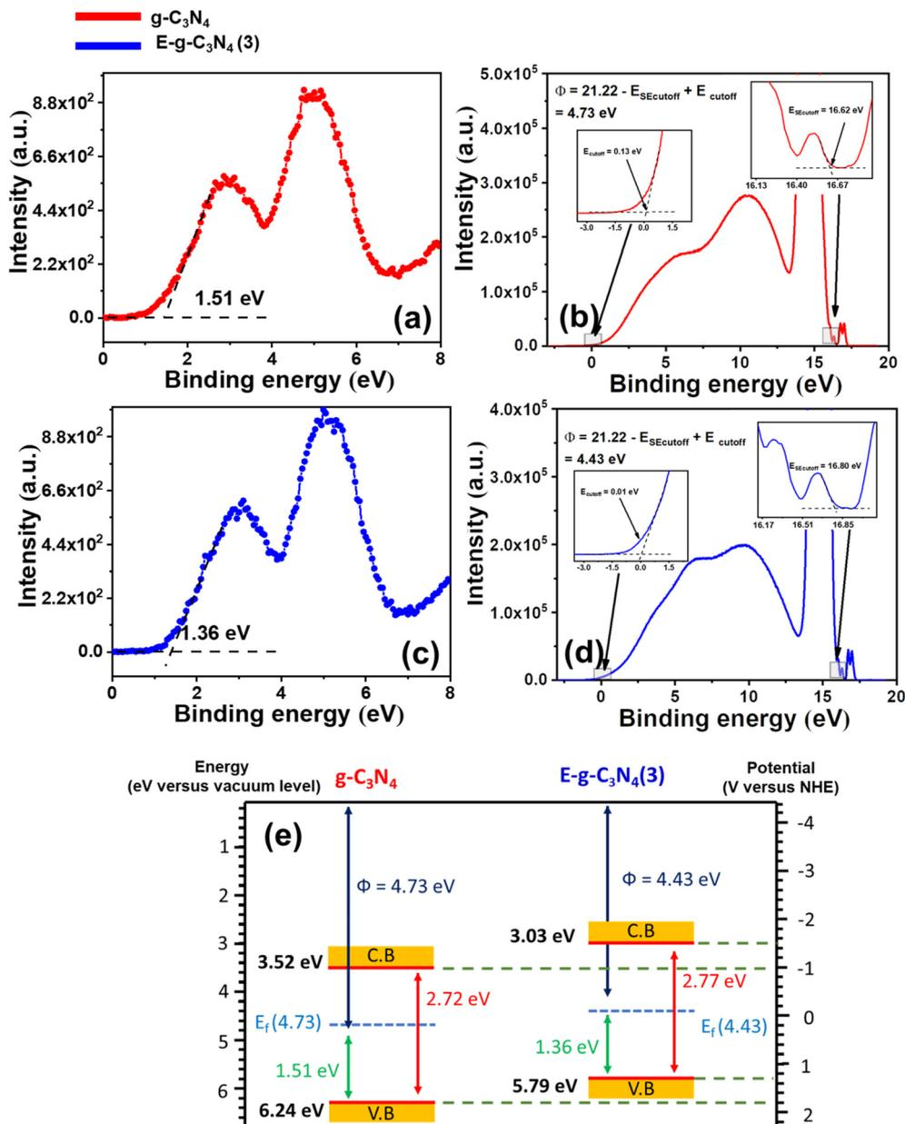
Fig. 6 (a) VB-XPS spectrum of g-C<sub>3</sub>N<sub>4</sub>, (b) UPS spectrum of g-C<sub>3</sub>N<sub>4</sub>, (c) VB-XPS spectrum of E-g-C<sub>3</sub>N<sub>4</sub>(3), (d) UPS spectrum of E-g-C<sub>3</sub>N<sub>4</sub>(3), and (e) band structures of g-C<sub>3</sub>N<sub>4</sub> and E-g-C<sub>3</sub>N<sub>4</sub>(3).
