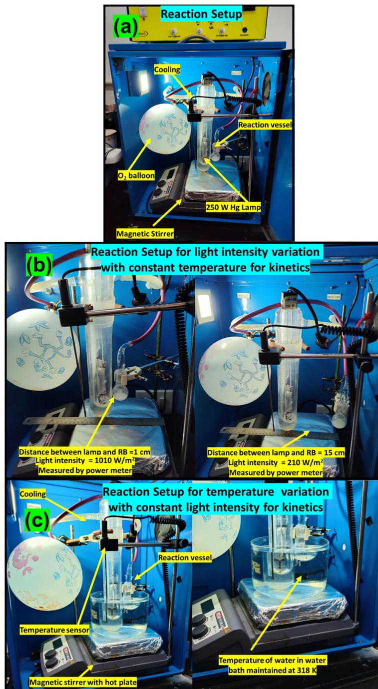
**Fig. 1** The digital image of the photocatalytic reactor and reaction setup for photocatalytic toluene oxidation (a) with constant temperature and light intensity, (b) with a variation of light intensity at a constant temperature, and (c) with a variation of temperature with constant light intensity.
