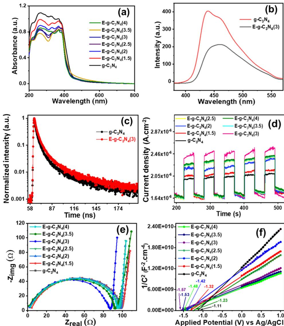
Fig. 5 (a) DRUV-vis spectra of pristine  $g\text{-C}_3\text{N}_4$  and exfoliated catalysts, (b) photoluminescence spectra of  $g\text{-C}_3\text{N}_4$  and  $\text{E-g-C}_3\text{N}_4(3)$ , (c) photoluminescence decays of pristine  $g\text{-C}_3\text{N}_4$  and exfoliated  $\text{E-g-C}_3\text{N}_4(3)$ , (d) transient photocurrent ( $i$ - $t$ ) response of all the photocatalysts, (e) electrochemical impedance of all the photocatalysts, and (f) M-S plots for various photocatalysts.
