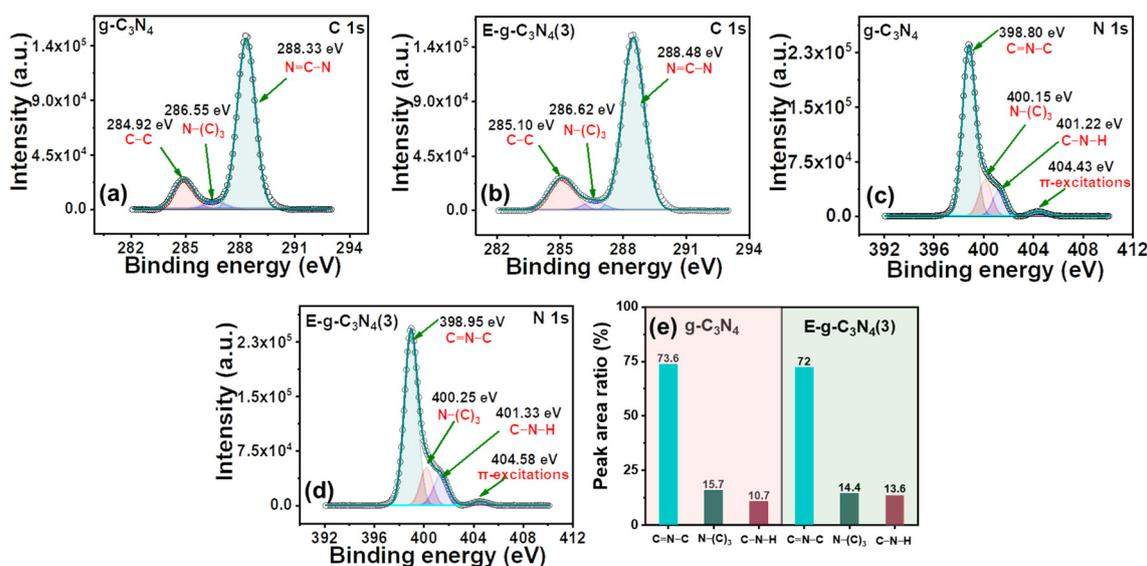
Fig. 4 (a) and (b) High-resolution C 1s XPS spectra of pristine g-C<sub>3</sub>N<sub>4</sub> and E-g-C<sub>3</sub>N<sub>4</sub>(3); (c) and (d) high-resolution N 1s XPS spectra of pristine g-C<sub>3</sub>N<sub>4</sub> and E-g-C<sub>3</sub>N<sub>4</sub>(3); (e) peak area ratio for various functional groups determined from (c) and (d).
