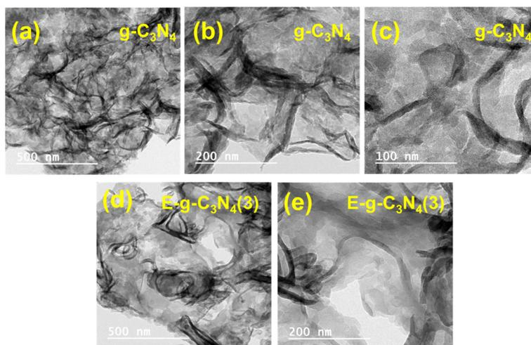
**Fig. 3** (a)–(c) TEM images of g-C<sub>3</sub>N<sub>4</sub>, and (d) and (e) TEM images of E-g-C<sub>3</sub>N<sub>4</sub>(3).
