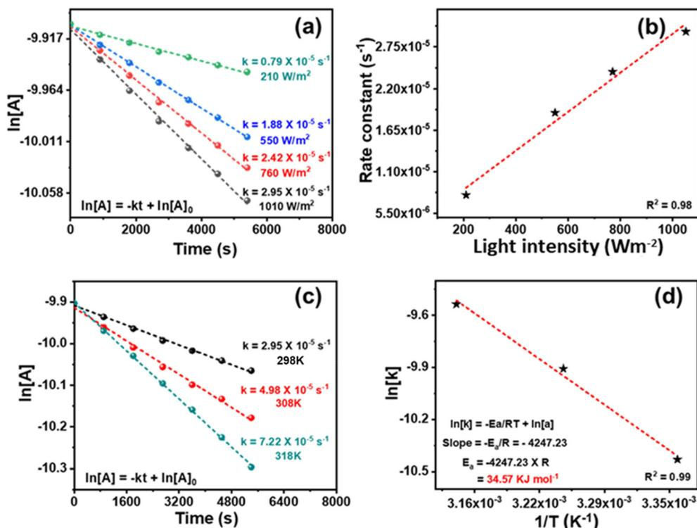
Fig. 8 (a) Kinetics plots of reaction at various intensities of light, (b) the dependence of rate constant ( $k$ ) on the light intensity at room temperature, (c) kinetic plots of the reaction at various temperatures (298 K, 308 K, and 318 K), and (d) Arrhenius equation plot for  $E_a$  calculation.
