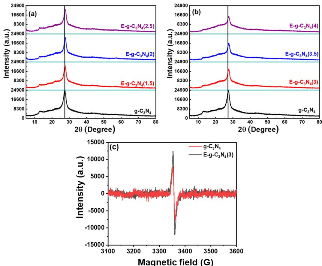
Fig. 2 (a and b) Powder XRD patterns, and (c) EPR spectra of pristine g-C<sub>3</sub>N<sub>4</sub> and E-g-C<sub>3</sub>N<sub>4</sub>(3).
