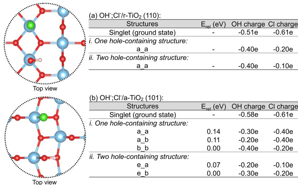
Fig. 8 Hydroxyl and chloride anions co-adsorption over r-TiO<sub>2</sub> (110) and a-TiO<sub>2</sub> (101) surfaces (a and b) and charges over hydroxyl and chloride when considering one (a.i and b.i) and two hole-containing structures (a.ii and b.ii). Computed charges in singlet (ground) state OH<sup>-</sup>,Cl<sup>-</sup>/r-TiO<sub>2</sub> (110) and OH<sup>-</sup>,Cl<sup>-</sup>/a-TiO<sub>2</sub> (101) are also given for comparison.
