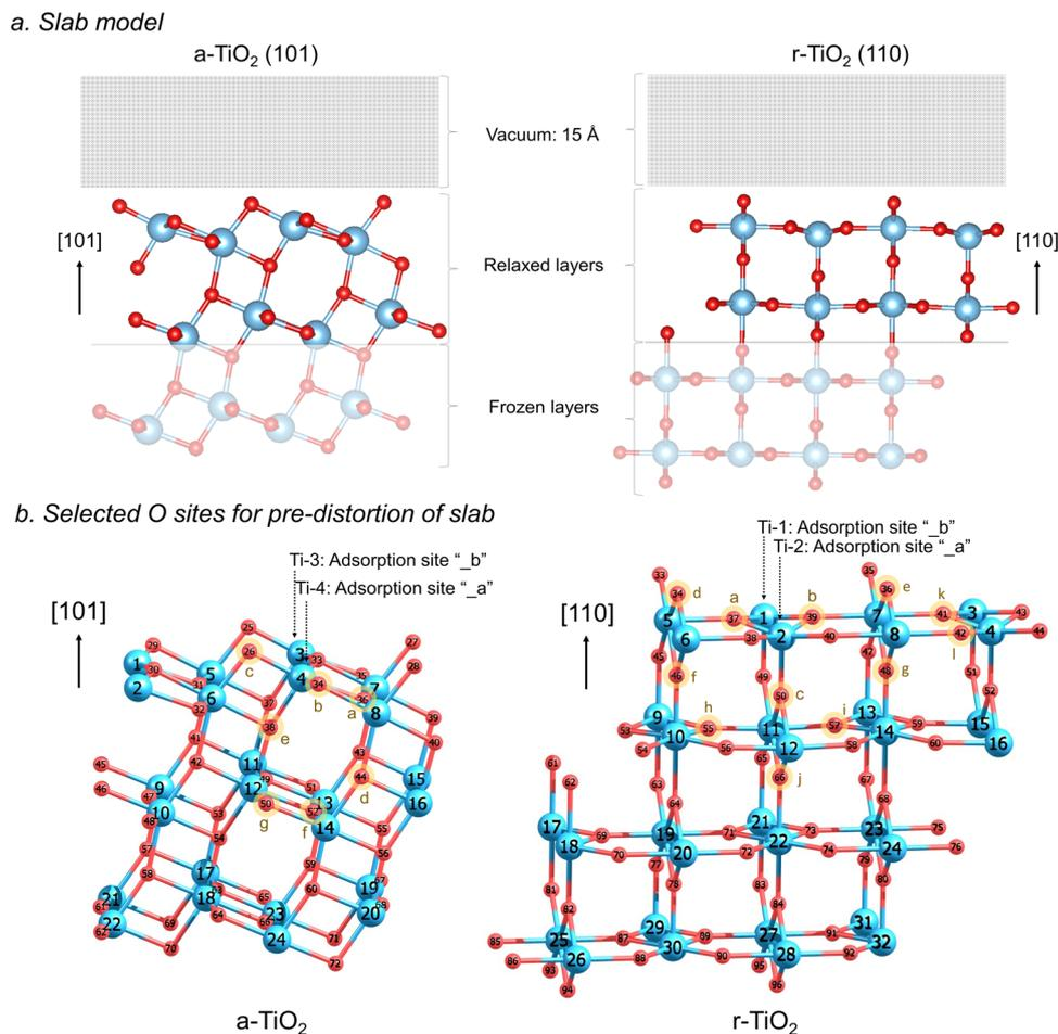
Fig. 1 Slab models used for  $r\text{-TiO}_2$  (110) and  $a\text{-TiO}_2$  (101) surface simulations (a) and selected O sites considered in the pre-distortion of  $r\text{-TiO}_2$  (110) and  $a\text{-TiO}_2$  (101) ionic structures (b). Alternative adsorption sites and number label of each atom are additionally shown.
