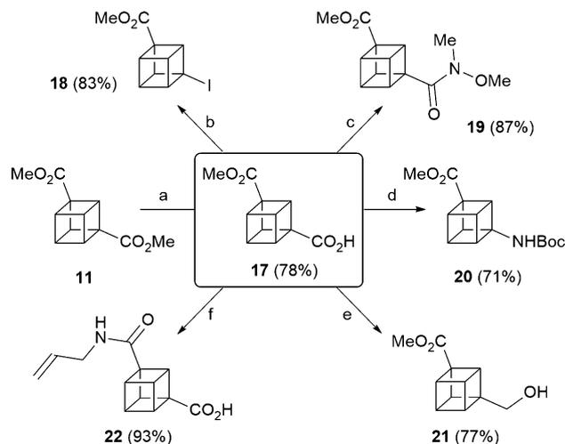
**Scheme 3** Selected synthetic manipulations of **17** to give five novel 1,3-disubstituted cubane derivatives. <sup>a</sup>NaOH (aq), MeOH <sup>b</sup>PhI(OAc)<sub>2</sub>, I<sub>2</sub>, C<sub>6</sub>H<sub>6</sub>, reflux <sup>c</sup>CDI, MeNH(OMe)-HCl, CH<sub>2</sub>Cl<sub>2</sub> <sup>d</sup>DPPA, Et<sub>3</sub>N, <sup>e</sup>tBuOH, reflux <sup>f</sup>BH<sub>3</sub>·SMe<sub>2</sub>, THF, 0 °C to rt <sup>g</sup>Allylamine, reflux. CDI = carbonyldiimidazole, DPPA = diphenylphosphoryl azide.
