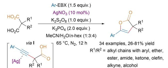
Scheme 34 Ag-catalyzed monodecarboxylative alkynylation–lactonization of malonic acid derivatives.
