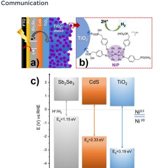
Fig. 1 (a) Schematic diagram of Sb<sub>2</sub>Se<sub>3</sub>/CdS/TiO<sub>2</sub>-meso/NiP hybrid photocathode. (b) Chemical structure of NiP catalyst molecular catalyst, panel a and b are not drawn to scale. (c) Equilibrium band alignment diagram of  $Sb_2Se_3/CdS/TiO_2$  heterojunction based on  $VBM^{11}$  and  $E_0$ measured separately for each layer (Fig. S2.1, ESI†), note that NiP redox couple is pH independent.21
