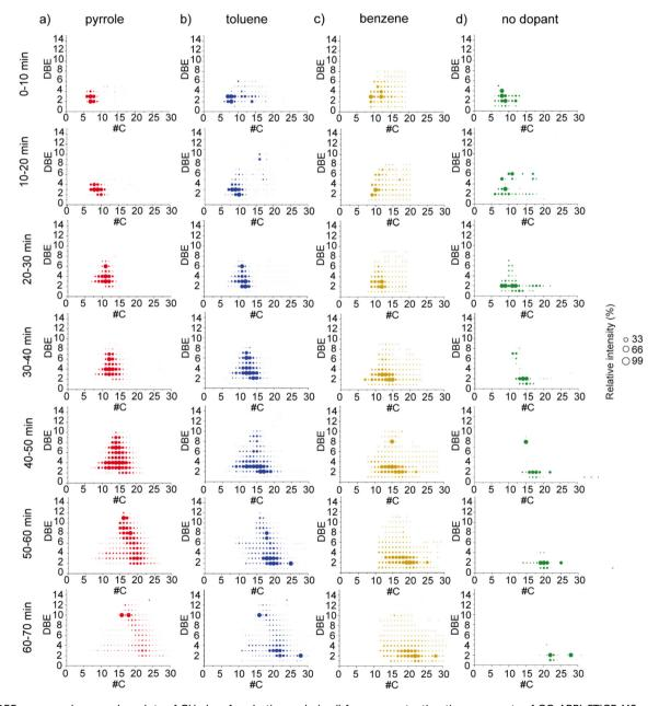
Fig. 5 DBE versus carbon number plots of CH class for plastic pyrolysis oil for seven retention time segments of GC-APPI-FTICR MS experiments with (a) pyrrole (red), (b) toluene (blue), (c) benzene (yellow), and (d) no dopant (green) for the CH class. The relative intensity was normalized for each DBE versus the carbon number plot.
