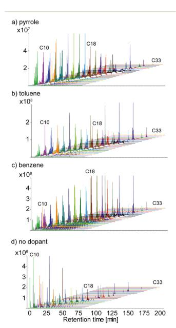
Fig. 6 Extracted ion chromatograms (EIC) of CH species with DBE value of 2 in ascending order for plastic pyrolysis oil with (a) pyrrole, (b) toluene, (c) benzene, and (d) no dopant. The EIC was obtained with a precision of around 1 mDa on the selected  $100-500 \ m/z$  value.
