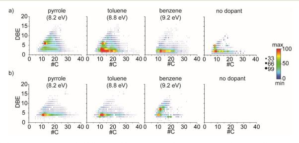
Fig. 4 DBE versus carbon number plots for (a) CH class and (b) N<sub>1</sub> class corresponding respectively to areas 2 and 1 of the 2D maps.
