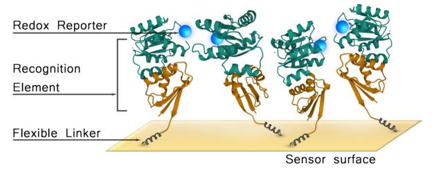
Fig. 1 Scheme illustrating the three main components of protein-based electrochemical biosensors: the recognition elements engineered within a redox reporter and attached to an electrode surface using a flexible linker.
