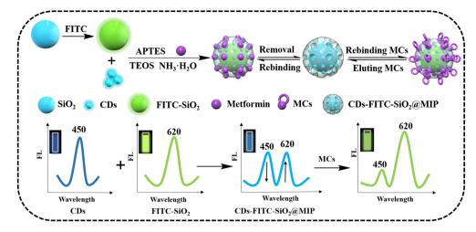
Fig. 1 Schematic illustration of the construction procedure and possible mechanism of the CDs-FITC-SiO₂@MIP sensor to detect MCs.
