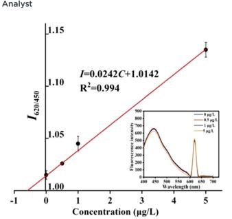
Fig. 8 The plot (n=3) of change in the fluorescence ratios against different MC-RR concentrations. The inset shows the fluorescence spectra for the determination of MC-RR in the water samples from Binhai Lake by the standard addition method. The concentrations of MC-RR were 0, 0.5, 1, and 5  $\mu$ g L<sup>-1</sup>.
