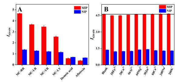
Fig. 6 Selectivity of CDs-FITC-SiO<sub>2</sub>@MIP and CDs-FITC-SiO<sub>2</sub>@NIP (A). The fluorescence response of CDs-FITC-SiO<sub>2</sub>@MIP and CDs-FITC-SiO<sub>2</sub>@NIP towards various interfering metal ions (B).
