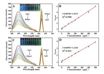
Fig. 5 The fluorescence spectra of the CDs-FITC-SiO<sub>2</sub>@MIP solution in response to a series of concentrations: MC-RR (A) and MC-LR (C), and the linear relationships for CDs-FITC-SiO<sub>2</sub>@MIP (B and D) ( $\lambda_{\rm ex}$  = 310 nm). The inset shows the images of the fluorescence colors of the corresponding solution under a 365 nm UV lamp. The error bar indicates three individual experiments.
