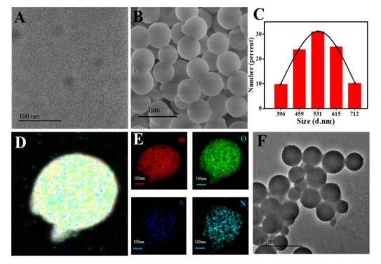
Fig. 3 The TEM image of the synthesized CDs (A), the SEM image of the synthesized FITC-SiO<sub>2</sub> nanocomposites (B), the diameter distributions of the FITC-SiO<sub>2</sub> nanocomposites (C), the HAADF-STEM image of the synthesized FITC-SiO<sub>2</sub> nanocomposites (D), the HAADF-STEM elemental mapping showing the presence of Si, O, S and N (E), and the TEM image of the synthesized CDs-FITC-SiO₂@MIP nanocomposites (F).
