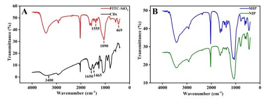
Fig. 4 FTIR spectra of the FITC-SiO<sub>2</sub>@MIP nanocomposites (red line) and CDs (black line) (A). FTIR spectra of the CDs-FITC-SiO<sub>2</sub>@MIP nanocomposites (blue line) and CDs-FITC-SiO<sub>2</sub>@MIP nanocomposites (green line) (B).
