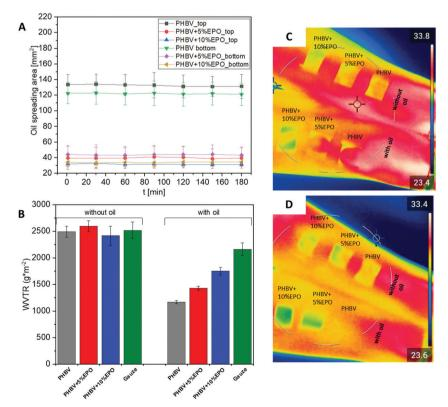
Fig. 6 Oil spreading area (A) on the PHBV electrospun fibers and blends with EPO over 3 h. (B) Water vapor and (C and D) heat transmission rates through the PHBV, PHBV + 5%EPO, and PHBV + 10%EPO electrospun fibers and samples with an additional 30  $\mu$ l EPO.
