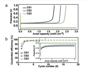
Fig. 3 (a) Initial Li deposition and stripping voltage profiles for the CS1, CS2, and CS3 composite anodes. (b) Variation in the coulombic efficiency during repeated Li plating and stripping of the CS1, CS2, and CS3 composite anodes. (Inset) Enlarged voltage profiles of the initial Li deposition.
