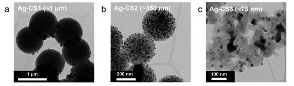
Fig. 5 TEM images of (a) Ag-CS1, (b) Ag-CS2, and (c) Ag-CS3.
