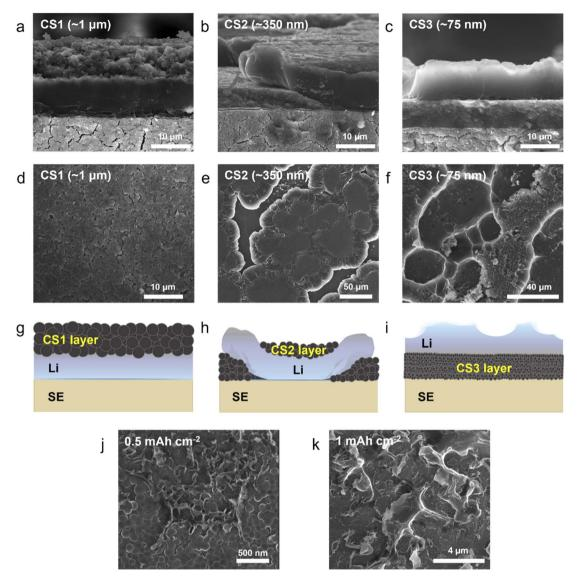
Fig. 2 (a-c) Cross-sectional and (d-f) top-view SEM images and (g-i) schematic illustrations of the Li in CS composite anodes deposited to a capacity of 3 mA h cm<sup>-2</sup>. (a, d, and g) for CS1, (b, e, and h) for CS2, and (c, f, and i) for CS3. Top-view SEM images of Li deposits on the CS3 composite anode at capacities of (j) 0.5 and (k) 1 mA h cm<sup>-2</sup>.
