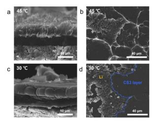
Fig. 4 (a and c) Cross-sectional and (b and d) top-view SEM images of the Li deposited CS3 composite anode plated to a capacity of 3 mA h cm $^{-2}$  at (a and b) 45 °C and (c and d) 30 °C.
