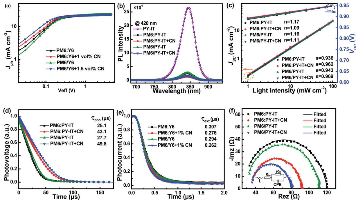
Fig. 3 (a)  $J_{ph}$ – $V_{eff}$  curves of all-PSCs. (b) Photoluminescence spectra of the PY-IT film, and PM6:PY-IT and PM6/PY-IT blend films under 420 nm light excitation. (c)  $J_{sc}$ – $P_{light}$  and  $V_{oc}$ – $P_{light}$  curves of all-PSCs. (d) Transient photovoltage curves of all-PSCs. (e) Transient photocurrent curves of all-PSCs. (f) Nyquist plots and the equivalent circuit of all-PSCs.
