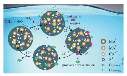
Fig. 16 The schematic reaction of organic dyes in the presence of the MoCoOS catalyst and NaBH<sub>4</sub>.
