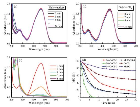
Fig. 9 (a) Reduction of MO with only MoCoOS-2. (b) Reduction of MO with only NaBH<sub>4</sub>. (c) Reduction of MO with MoCoOS-2 and NaBH<sub>4</sub>. (d) Reduction of MO with Mo(S,O), Co(O,S), and MoCoOS catalysts in the presence of NaBH<sub>4</sub>.
