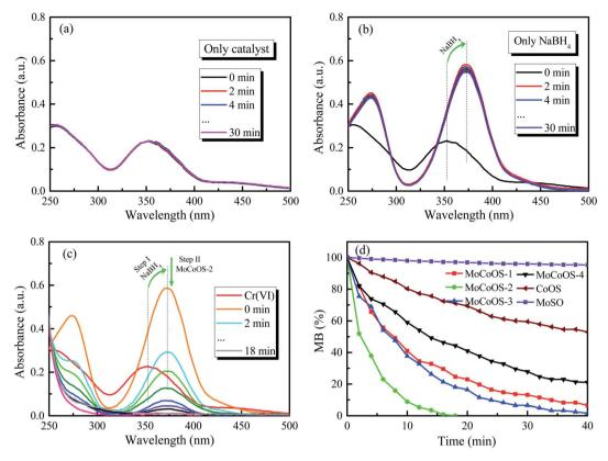
Fig. 12 (a) Reaction of Cr(vi) with only MoCoOS-2, (b) reaction of Cr(vi) with only NaBH<sub>4</sub>, (c) reduction of Cr(vi) with MoCoOS-2 and NaBH<sub>4</sub>, (d) reduction of Cr(vI) with Mo(S,O), Co(O,S), and MoCoOS catalysts in the presence of NaBH<sub>4</sub>.
