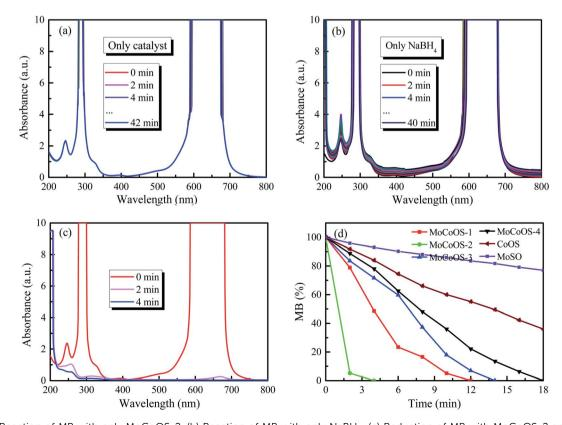
Fig. 10 (a) Reaction of MB with only MoCoOS-2 and NaBH<sub>4</sub>. (d) Reduction of MB with MoCoOS-2 and NaBH<sub>4</sub>. (d) Reduction of MB with Mo(S,O), Co(O,S), and MoCoOS catalysts in the presence of NaBH<sub>4</sub>.
