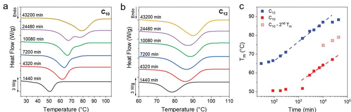
Fig. 3 (a and b) DSC of  $C_{10}$  and  $C_{12}$  after long time crystallization at room temperature. A monotonic increase in the  $T_m$  is evident from the rightward shift of the melting curve. DSC data for less than 1 day of crystallization time can be found in Fig. S2 (ESI†). (c) A plot of  $T_m$  vs. time shows similar slopes for the two networks. The 7, 17 and 30 day samples of  $C_{10}$  show two melting peaks, the lower one shown as solid squares and the higher peak as crossed squares.
