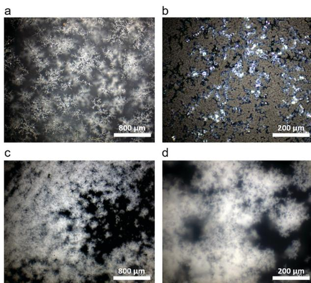
Fig. 6 (a) and (b) Dendritic structures are seen in other locations of the same  $C_{10}$  sample along with the crystals shown in Fig. 5. (c) and (d) After annealing at 50 °C for 2 days the dendrites span the entire crystal domain and the spherulites are no longer visible.
