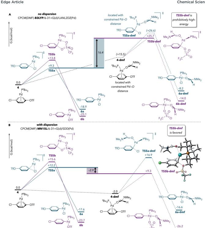
Fig. 2 Effect of dispersion on the stability of DMF-coordinated oxidative addition transition structures. Calculations were performed (A) without dispersion or (B) with dispersion. Free energy values are corrected for concentration (DMF: Pd = 765: 1) and are reported after applying Cramer and Truhlar's<sup>29</sup> and Head-Gordon's<sup>30</sup> quasi-harmonic approximations to vibrational entropy and enthalpy, respectively.<sup>31,32</sup>
