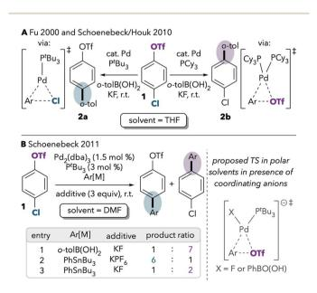
Scheme 1 Seminal reports on the effects of (A) ligands and (B) solvents on the selectivity of cross-coupling of a chloroaryl triflate.<sup>5,7,9</sup>
