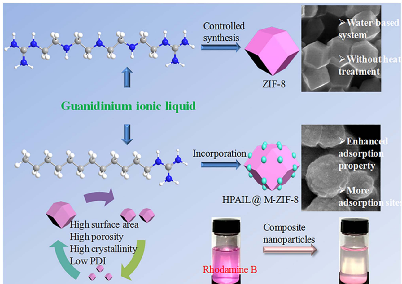
Fig. 4 HPAIL@Meso-ZIF-8 composite for the removal of RhB dye. Reproduced with permission from ref. 89 Copyright ©2022, Elsevier.
