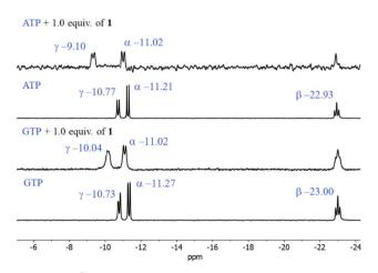
Fig. 3 Partial  $^{31}$ P NMR spectra (121.5 MHz, 25  $^{\circ}$ C) of sodium salts of ATP and GTP (3.0 mM) in the presence of 1.0 equiv. of 1 in  $D_2O$  at pD=7.0 (10 mM MOPS).
