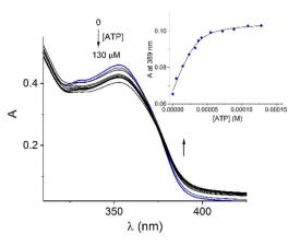
Fig. 5 Spectrophotometric titration experiment of buffered aqueous solution of 1 (40  $\mu\text{M})$  upon the addition of increasing amounts of ATP at pH = 7.0 (10 mM MOPS, 25 °C). Inset: shows the profile of absorbance at 389 nm for increasing amounts of ATP. The solid lines were obtained by fitting the experimental data to a 1 : 1 model. The ionic strength was adjusted to 0.05 M of NaCl.
