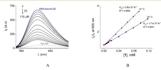
Fig. 9 (A) Fluorescence spectra ( $\lambda_{ex} = 520$  nm) of DNA-EB upon the addition of increasing amounts of 1 at pH = 7.0 (10 mM MOPS, 25 °C). DNA and EB total concentrations are 250 μM and 50 μM, respectively. The ionic strength was adjusted to 50 mM of NaCl. (B) S-V plots for the quenching of system DNA-EB by 1 at 25 and 37 °C.
