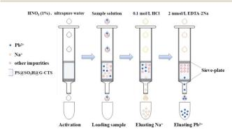
Fig. 1 The separation processes of SPE column.
