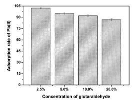
Fig. 3 Effects of different crosslinkers (left) and glutaraldehyde concentrations (right) on the adsorption of Pb(III) by chitosan modified PS microspheres.
