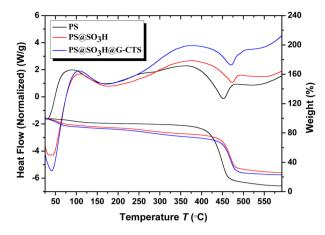
Fig. 6 TGA and DSC of PS, PS@SO3H and PS@SO3H@G-CTS.
