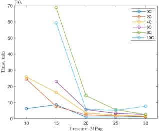
Fig. 7 The time required for the 1 ppm O-MWCNT-methane-water system to reach (a) 200 mPa s and (b) 500 mPa s from the onset of hydrate formation at various pressures.
