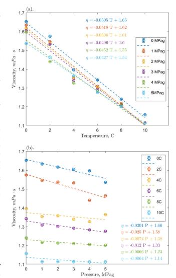
Fig. 4 Effect on the measured viscosity of the 1 ppm O-MWCNTmethane-water system of (a) temperature and (b) pressure; error bars represent the 95% confidence intervals on the measured mean viscosity.
