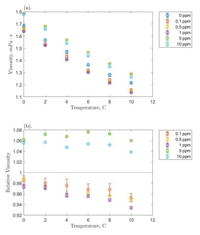
Fig. 2 Temperature effect on the measured viscosity of the O-MWCNT-water system studied. This includes (a) the absolute viscosity and (b) the relative viscosity compared to a pure water baseline. Bars represent the 95% confidence intervals on the data, which are very small.
