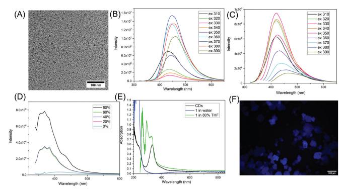
Fig. 4 (A) A representative TEM image of the CDs; (B) fluorescence spectra of CDs; (C) fluorescence spectra of 1 excited at 330 nm in mixed solvents of DMSO and THF, with the percentage indicating the THF%; (E) UV-vis absorption of CDs as well as 1 in water and in a mixed solvent of 80% THF and 20% DMSO; (F) a fluorescent macroscopic image of solid 1 particles (excitation 360–380 nm; emission 415 nm with longpass filter, scale bar is  $200 \mu m$ ).
