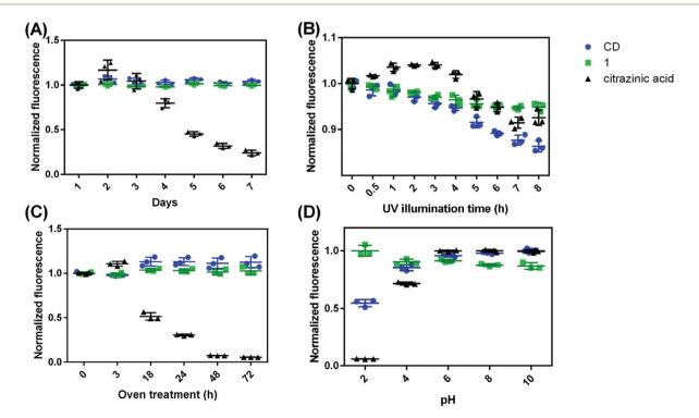
Fig. 6 Normalized fluorescence of CDs, 1, and citrazinic acid. (A) samples were dissolved in water at room temperature; (B) underwent 365 nm UV illumination; (C) underwent 50 °C oven treatment; and (D) in a series of pH conditions. Each treatment has 3 materials replicates, and the error bars show the standard deviation.
