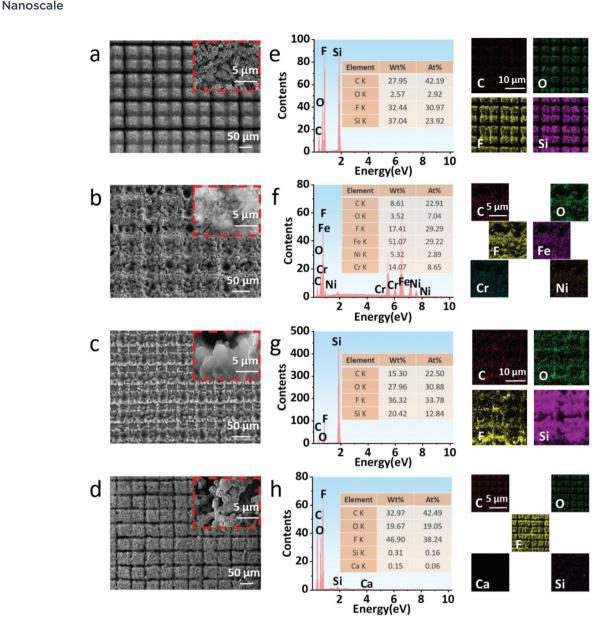
Fig. 2 (a-d) SEM images of quartz glass, stainless steel, silicon wafer, and paper after femtosecond laser ablation; (e-h) EDS spectra and elemental mapping of laser-treated quartz glass, stainless steel, silicon wafer, and paper, respectively.
