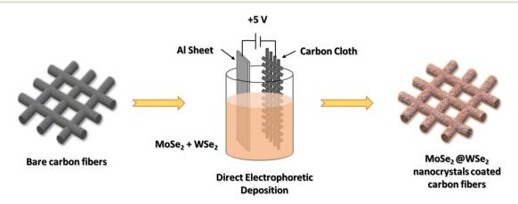
Fig. 1 Direct EPD of MoSe<sub>2</sub>@WSe<sub>2</sub> HS thin film on carbon cloth substrate.
