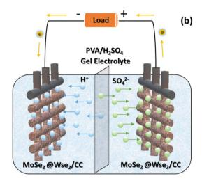
Fig. 8 The schematic working mechanism of (a) hydrogen evolution and (b) FSSC-based on MoSe<sub>2</sub>@WSe<sub>2</sub> HS composite on CC.
