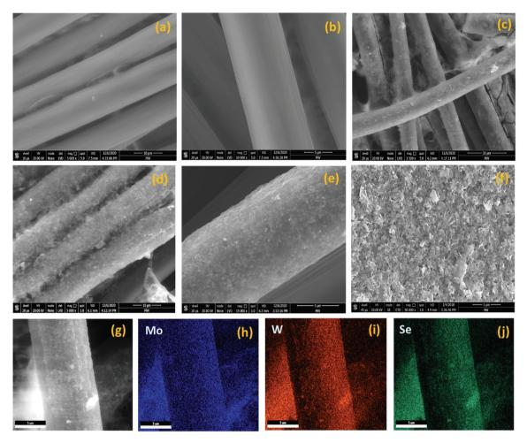
Fig. 5 (a) The schematic illustration of MoSe<sub>2</sub>@WSe<sub>2</sub> HS film deposition on carbon fiber cloth by EPD. SEM images of (b and c) bare carbon fibers and (d and e) MoSe<sub>2</sub>@WSe<sub>2</sub> HS-coated carbon fibers. (f-i) EDAX elemental mapping of MoSe<sub>2</sub>@WSe<sub>2</sub> HS on single CF.
