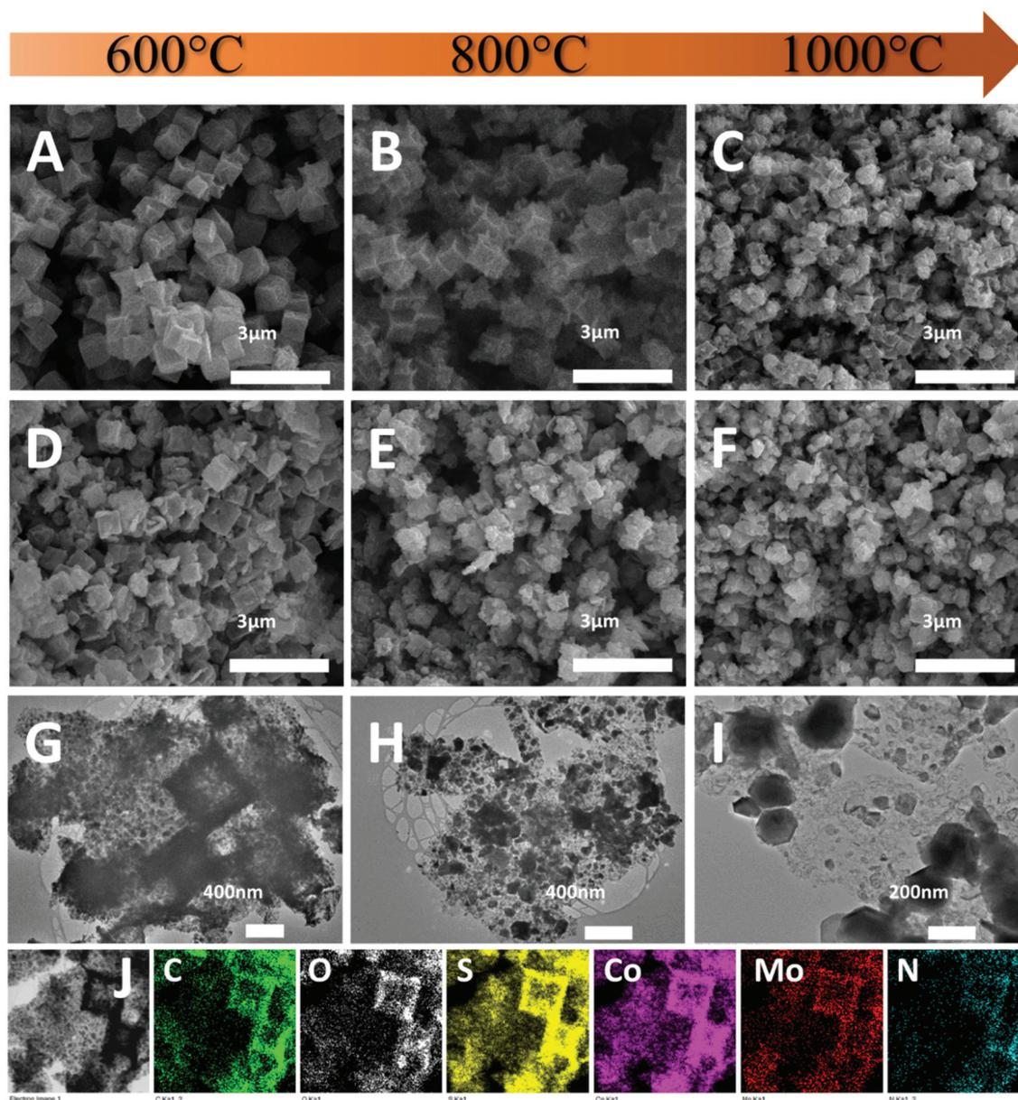
**Fig. 3** SEM images of (A) CoS-600, (B) CoS-800, (C) CoS-1000, (D) CoMoS-600, (E) CoMoS-800, and (F) CoMoS-1000; TEM images of (G) CoMoS-600, (H) CoMoS-800, and (I) CoMoS-1000 and (J) elemental mappings of CoMoS-600 obtained by TEM.
