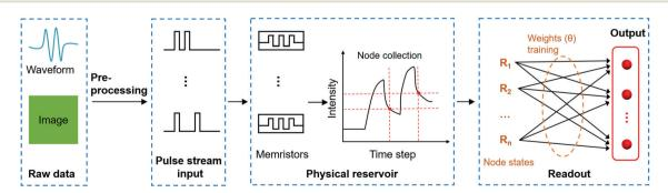
Fig. 2 Schematic of an information processing flow chart using a dynamic memristor-based RC system, consisting of the preprocessing of input signals, the memristor response, the collection of node states, readout, and the final output.
