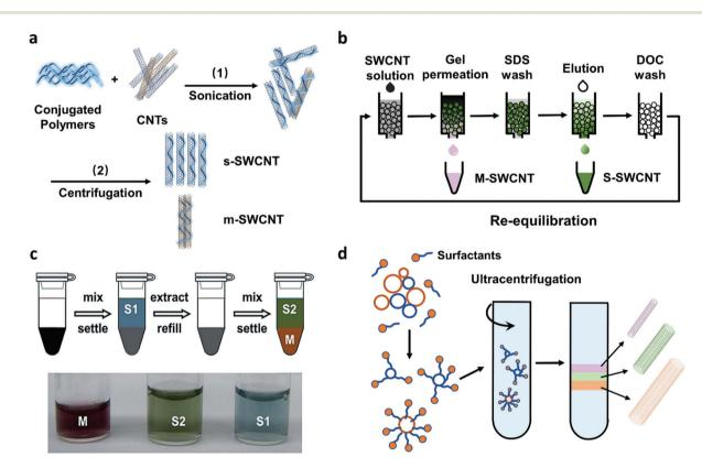
Fig. 1 Four solution-based post-growth separation methods. (a) Conjugated polymer wrapping (CPW). (b) Gel permeation chromatography (GC). (c) Aqueous two-phase extraction (ATPE). Reproduced with permission. 32 Copyright 2015, American Chemical Society. (d) Density gradient ultracentrifugation (DGU).
