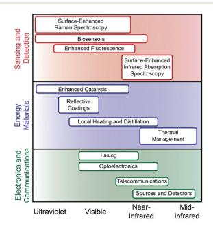
Fig. 1 Representation of functional versatility in plasmonic materials across the electromagnetic spectrum. The integration of non-archetypal plasmonic materials has greatly expanded the region of spectral activity and enhanced functionality in the areas of sensing and detection, energy materials, and electronics and communication.
