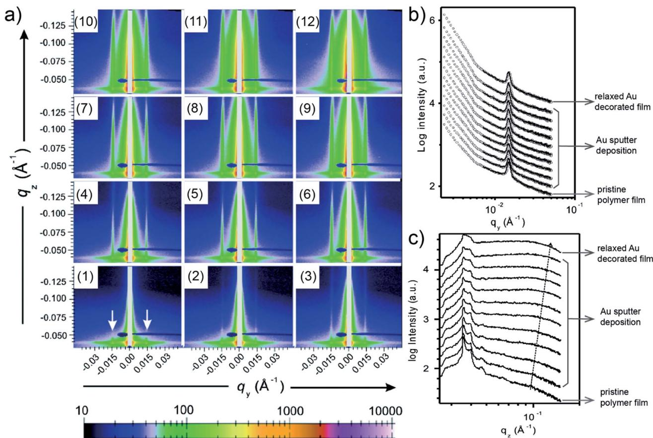
Fig. 8 (a) 2D GISAXS data of (a1) pristine phase-separated polymer thin film, (a2)–(a11) 10 repetitions of 6 s sputter deposition onto the polymer film, and (a12) polymer film with 4.3  $\text{\AA}$ -thick deposited Au after 10 h relaxation. (b) Horizontal and (c) vertical line cuts of the 2D GISAXS data. Reproduced with permission.<sup>59</sup> Copyright 2008 American Chemical Society.
