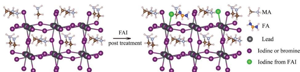
Fig. 6 Schematic illustration of the filling of  $I^-$  and  $MA^+$  vacancies in the perovskite films by the FAI post-treatment process<sup>133</sup> [Reprinted with permission. Copyright (2018) American Chemical Society].
