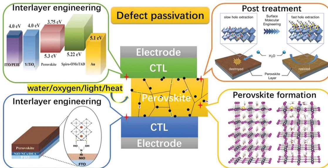
Fig. 7 Schematic showing the general defect passivation strategies for PSCs [Reproduced from Royal Society of Chemistry].<sup>137</sup>
