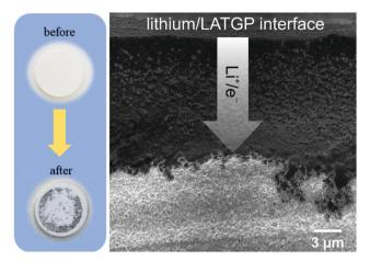
**Fig. 1** LATP pellets before and after the contact with the Li metal chip and SEM cross-section image of LATGP after contact with Li metal.<sup>75</sup>
