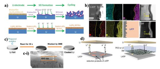
Fig. 2 Illustration of the deposition of various inorganic protective layers on LATP and their TEM and SEM images: (a) explanation of the role of the SEI layer; 88 (b) TEM-EDS of Li<sub>3</sub>PO<sub>4</sub> deposited LATP after 100 cycles; 89 (c) nanocomposite layer formation through the dropping of solution; (c-i) crosssectional view of the nanocomposite layer on LATP; 90 (d) scheme of BN and polymer combined thin layer on LATP. 91
